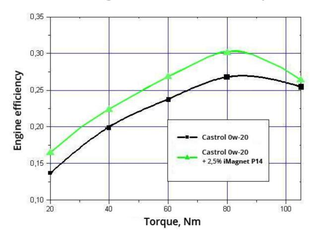
During the test, engine efficiency was increased by **10-12%** with the addition of **iMagnet P14** in comparison with the base oil.
