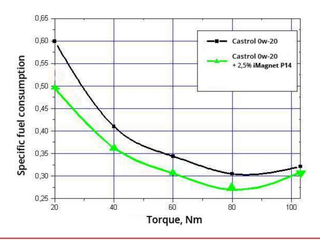
Fuel consumption reduced by **8-11,9%** (depending on the operating mode) due to adding of **iMagnet P14** into **Castrol Edge 0w-20** base oil.
