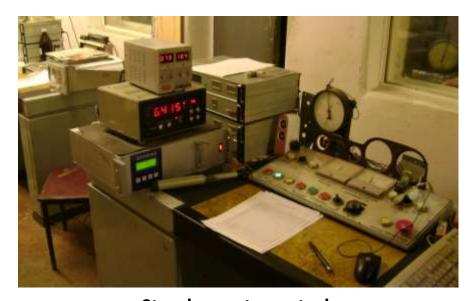
Stand remote control. Fuel flowmeter and gas analyzer
