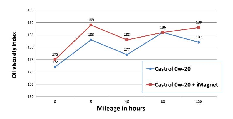
The oil viscosity index is increased with adding of iMagnet P14 which increases the protection of the engine over a wide range of operating conditions. Including extreme conditions (cold start and high rpm).
