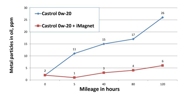
Reducing of engine wear was proved and the contamination of metal particles was reduced by 5 times during using of iMagnet P14.
